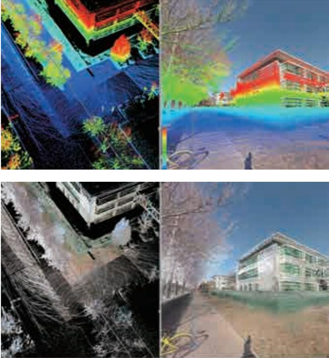
LiFuser-BP is GreenValley's self-developed data fusion software for LiBackpack Lidar scanning systems, including measurement, clipping, profile editing, coordinate transformation, export, and other tools.
