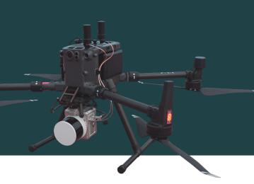
The LiAir X3C-H is a new compact high-performance UAV LiDAR system and is the upgraded version of the LiAir300 by GreenValley International. It adopts a new integrated design style and built-in high-resolution mapping camera,, providing higher performance and convenient operation for power-line inspection, topographic surveying, agricultural and forest monitoring, and more.
